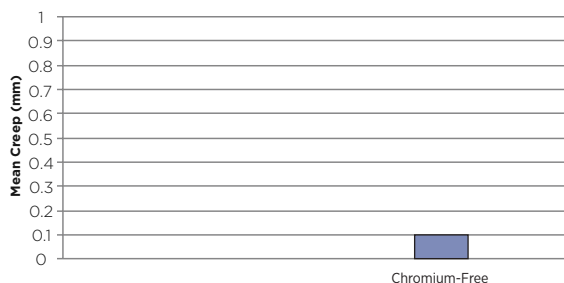
Figure 7: Sherwin-Williams Coil Coatings exposed test panels in Daytona Beach, Florida, comparing chromium-free primer to chromium primer. This coastal marine test site has very moist, warm air, strong UV rays and salt spray—a high corrosivity environment. Corrosion was measured, and creep was minimal—less than 1 mm on average. Furthermore, the scribe, face and tension bends gave good performance on the test panels.
