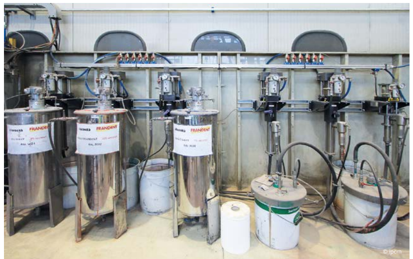
From top to bottom: The 4-stage pre-treatment tunnel, primed components, and the paint management unit.
