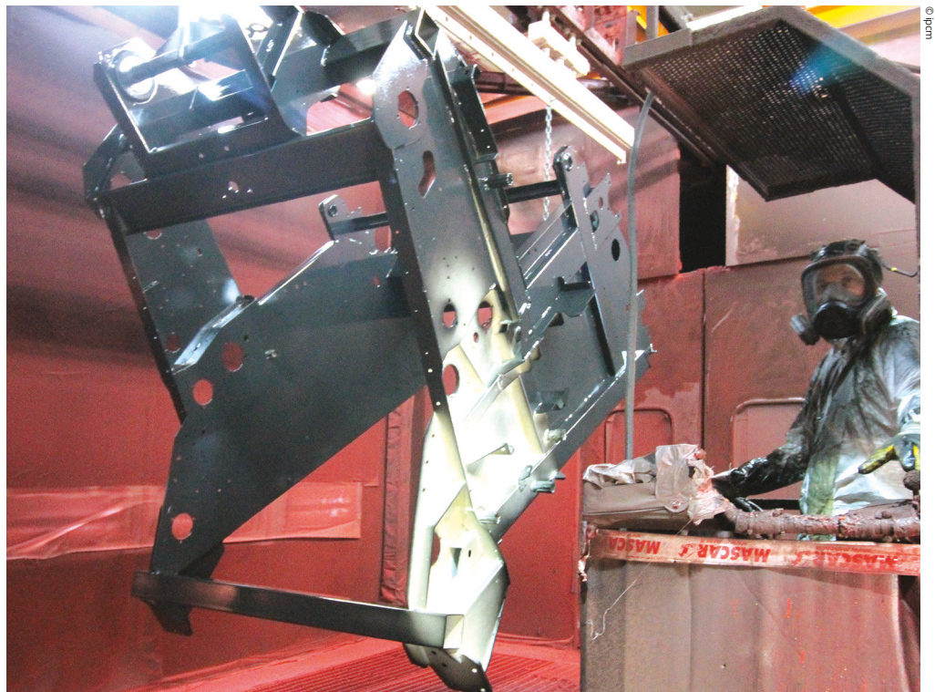
Figure 4: Manual top coat application.
