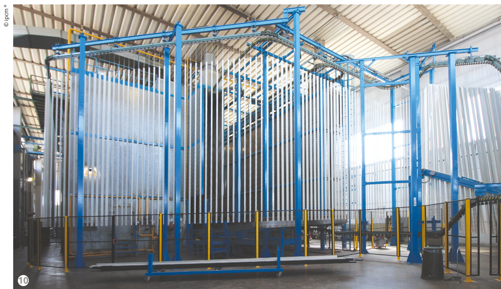
Figures 10 and 11: The storage buffer for cooling the profiles and the unloading area.
