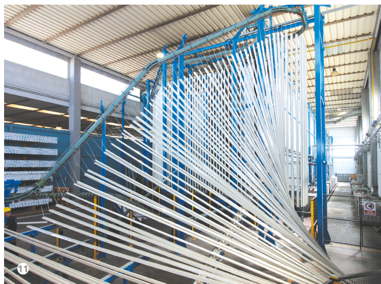
Figures 10 and 11: The storage buffer for cooling the profiles and the unloading area.
