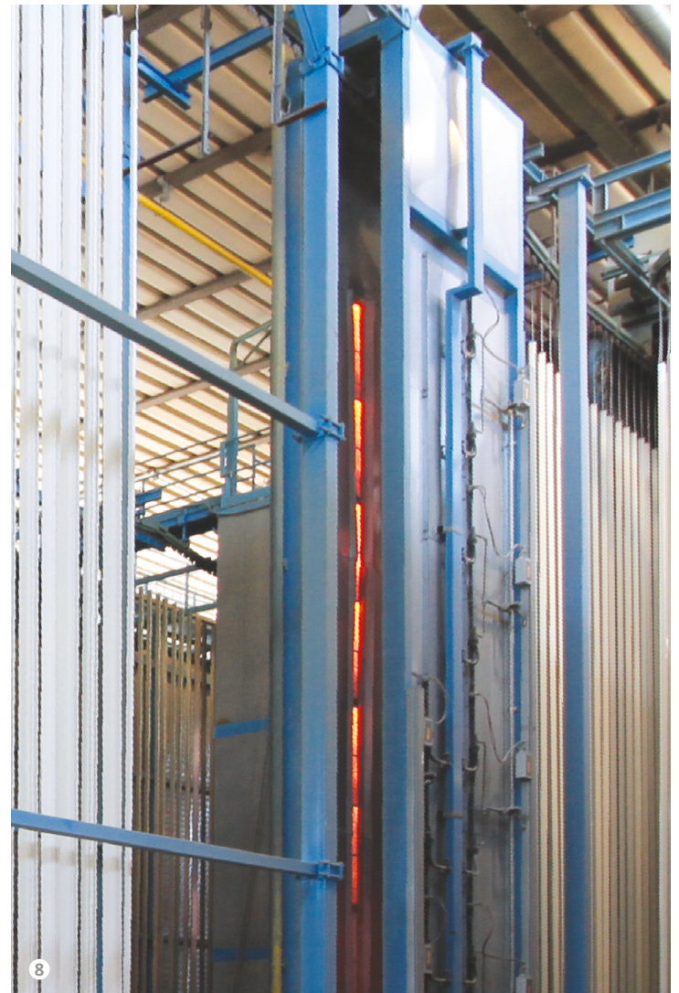
Figure 8: The IR gelling oven installed before the polymerisation oven for greater control over colour and contamination.
