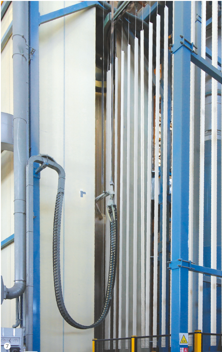
Figure 7: Trasmetal's coating booth paints the profiles with two OFB disks.
