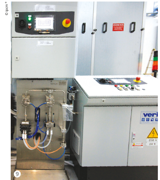
Figure 9: Verind's EcoDose 2K automatic system for the dosing and mixing of 2K coatings.
