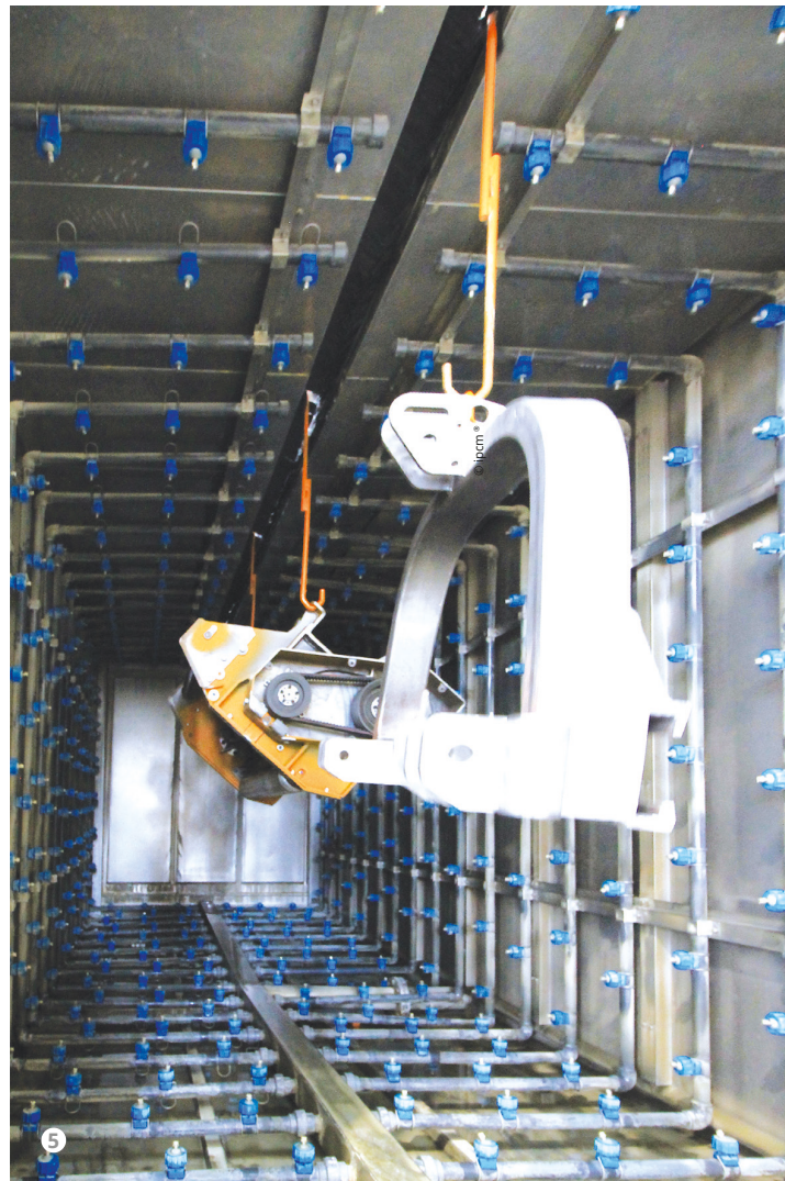
Figure 5: The 3-stage chemical pre-treatment process.
