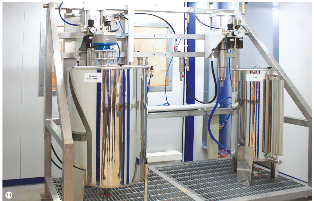
Figure 11: The feeding system of the primer application booth for manual station with Dürr pump.
