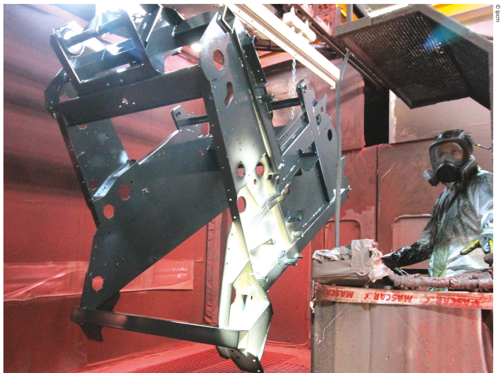
Figure 4: Manual top coat application.
