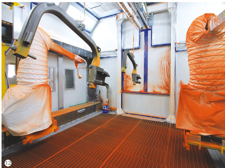
Figures 12 and 13: Gaiotto's GA25-P six-axis spraying robots.
