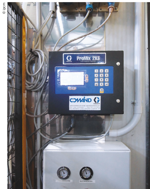
Figures 8 and 9: For the top coat application, Mascar installed the 2KS multi-component dosing system, which allows managing up to five colours but is expandable up to a maximum of thirty.
