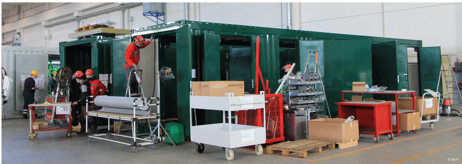
The assembly of components into a cogeneration plant.
