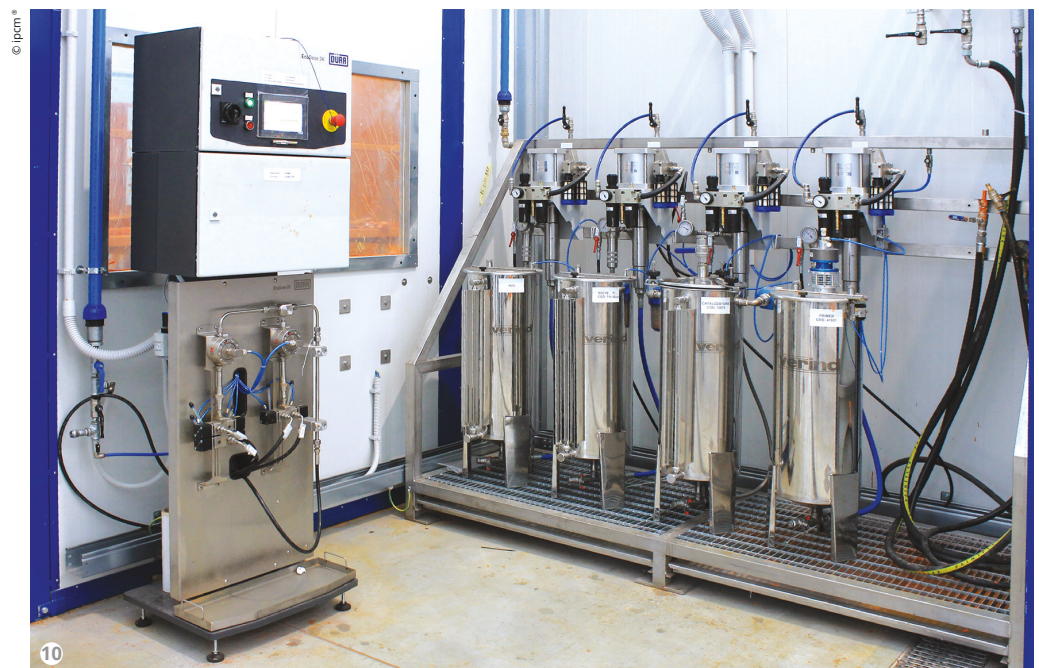
Figure 10: The coating management unit for manual station with Dürr pump.
