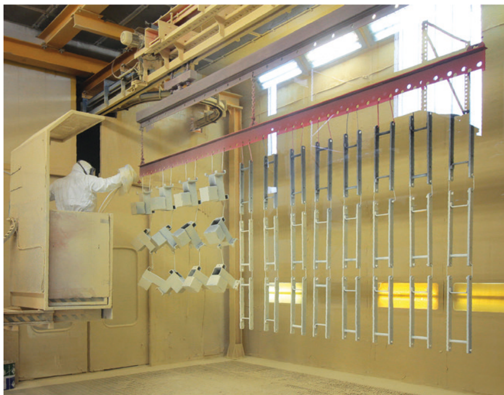
Figure 3: Manual primer application.
