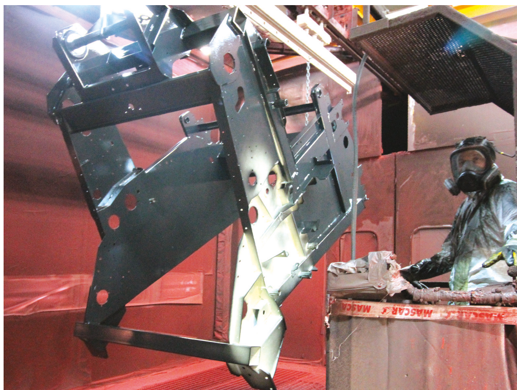
Figure 4: Manual top coat application.
