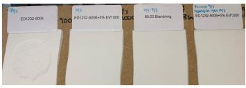
Usage time of the mix WB product and EV1000 is 24h. After 24h you can rework the old mix into a freshly mixed one in the ration 20:80 and keep the good performance just like you do with a 2C SB AC.
