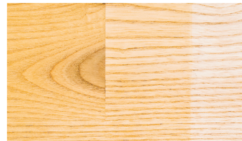
Untreated ash. Light-coloured wood yellows easily.
