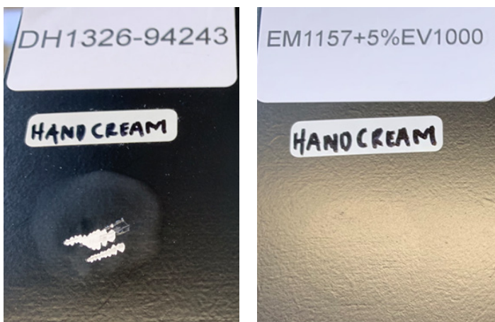
Picture 2 Usually EM1157 has a poor resistance to hand cream. Already after a few minutes it starts to dissolve, but with EV1000 it becomes so much better.
