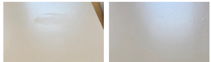
Picture 2 Usually EM1157 has a poor resistance to hand cream. Already after a few minutes it starts to dissolve, but with EV1000 it becomes so much better.
