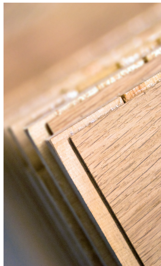
On each of the three panels the left side has been exposed to 100 hours of UV light, while the right side has been protected with aluminium foil to illustrate the original colour.
