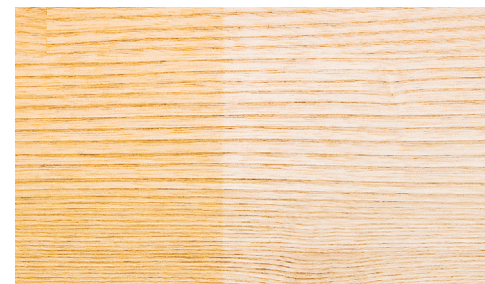
Ash coated with an ordinary non-yellowing UV system. Much of the yellowing comes from the wood itself.
