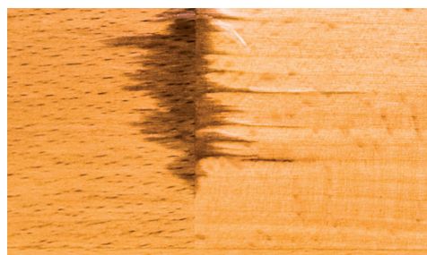
The picture on the top shows the effect after 30 mins. of water exposure for our hydrophobic edge protector. No damage can be seen. The picture on the bottom shows the same coating and substrate without edge protection. Severe damage can be seen.
