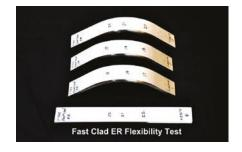
Note: The Fast  $Clad^{@}$  ER straps were bent to the approximate limit of the bend apparatus with no visible signs of failure.
