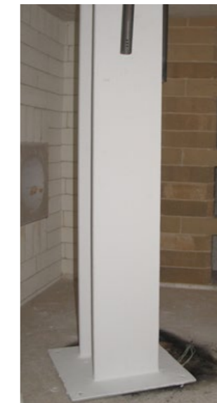
Fig. left: Coated test specimen before fire
