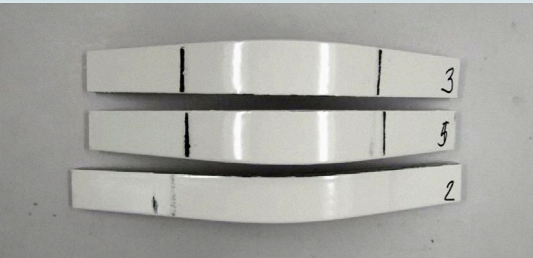
Figure 2: Dura-Plate 301W Flexibility samples after 4-point bend testing.
