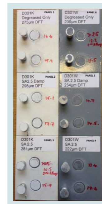
Figure 1: Dura-Plate 301W Panels after pull-off testing, showing failure mode and measured values. Figure also shows results from adhesion testing of a previous version of the Dura-Plate 301 series. Note: top dollies on Panels 1 and 6 show result after second attempt to pull. First attempt showed no failure, with dollies in place after interrupting pull-off when dial reach 25MPa (maximum)
