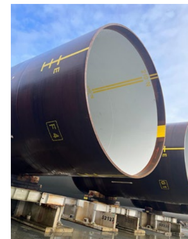
Monopiles are coated at the applicator facility, before being transferred to the docks and continuing their journey offshore.
