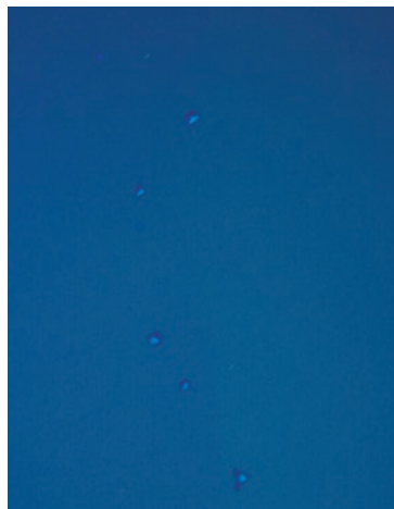
Pinholes are easy to identify under UV light inspection. No flashlight glare.
