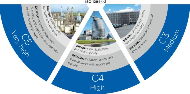
The corrosivity categories were restructured in the 2018 revised standard and now range from C1 to CX. Category CX (part 9 of the standard) refers to extremely corrosive environments, particularly offshore and industrial areas with extreme humidity.
