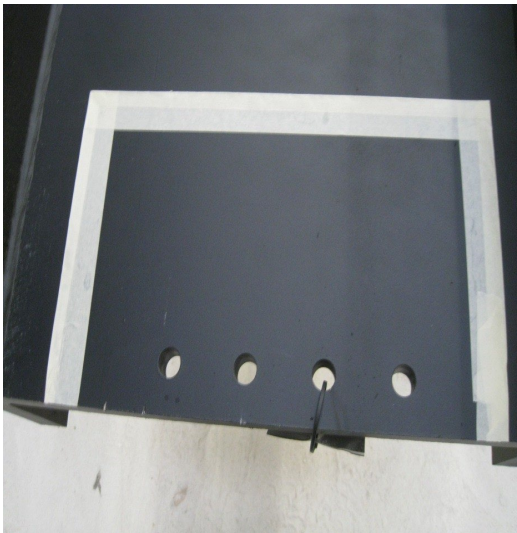
Single masked area/singled masked area with folded masking around edge, (multiple coat application).
