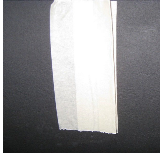
Folded masking tape on perimeter area/folded masking tape area with normal masking infill, (single coat application).
