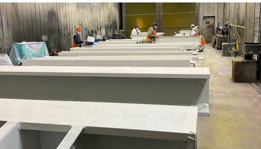
Figure 9. Puget Sound Coatings was able to fireproof an entire tier of the building – two full floors worth of structural steel that required intumescent coatings – within one of its industrial painting booths, helping the shop maintain high throughput for the project.
