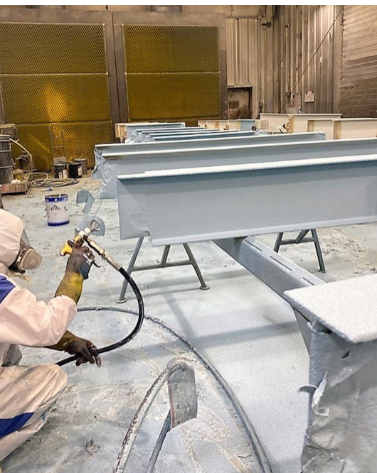
Figure 4. Puget Sound Coatings coated all the structural steel for 303 Battery inside its nearby 80,000-square-foot shop, ensuring greater quality control compared to performing the same work in a makeshift coatings booth erected at the construction site.
