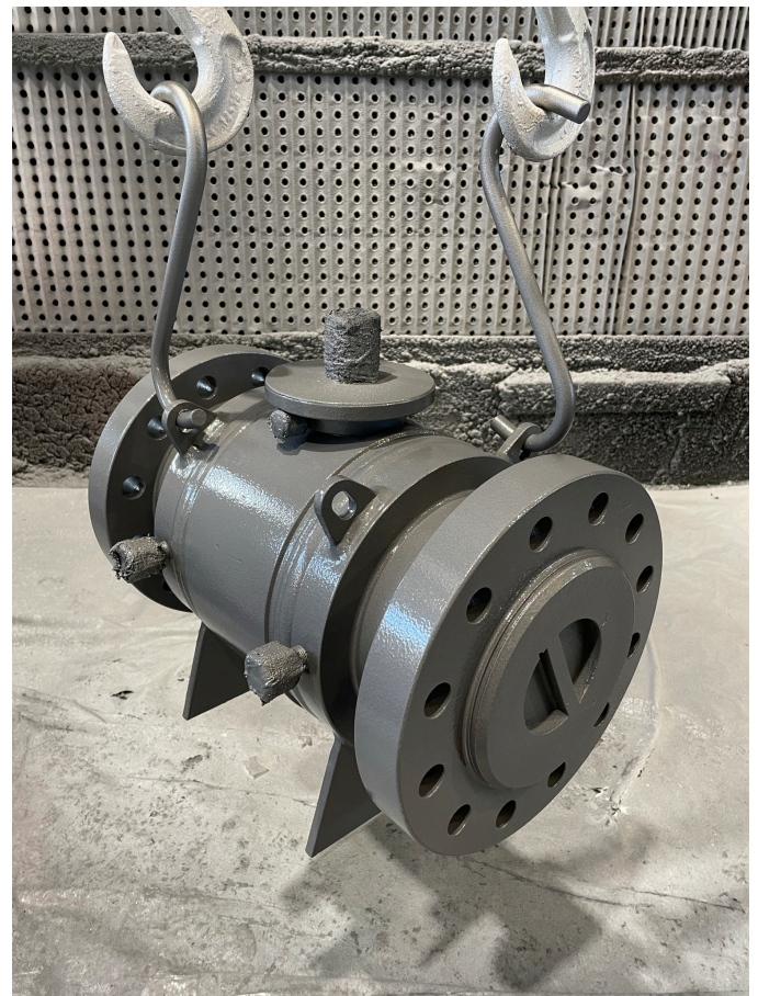
Figure 6. MIO-enhanced, high-solids alkylated amide epoxy coatings offer excellent protection from CUI on assets such as industrial valves used in LNG processing.
