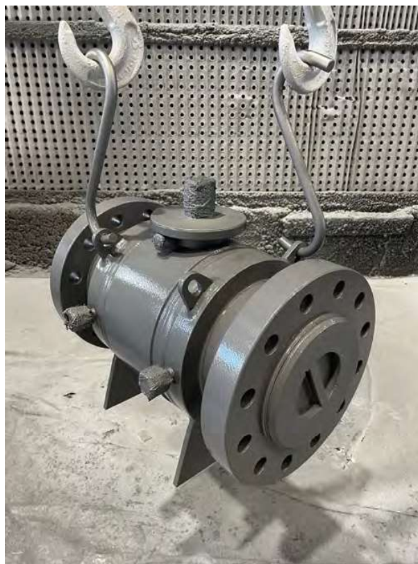
Figure 6. Applied to an industrial valve that will be insulated prior to service, an MIO-enhanced, high-solids alkylated amide epoxy coating will offer excellent protection from CUI.
