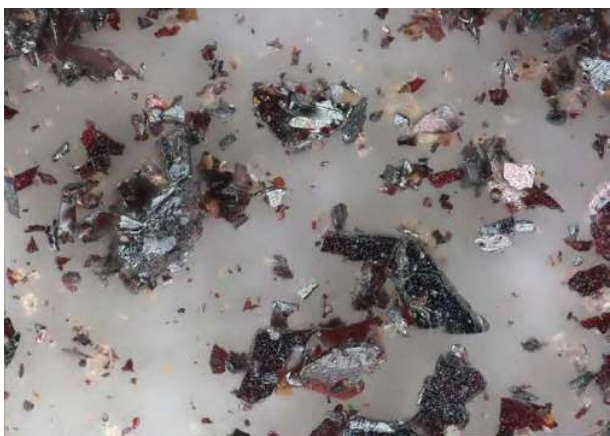
Figure 4. High concentrations of micaceous iron oxide (MIO) pigment embedded in liquid coatings adds durability against impacts, chemicals and corrosion.
