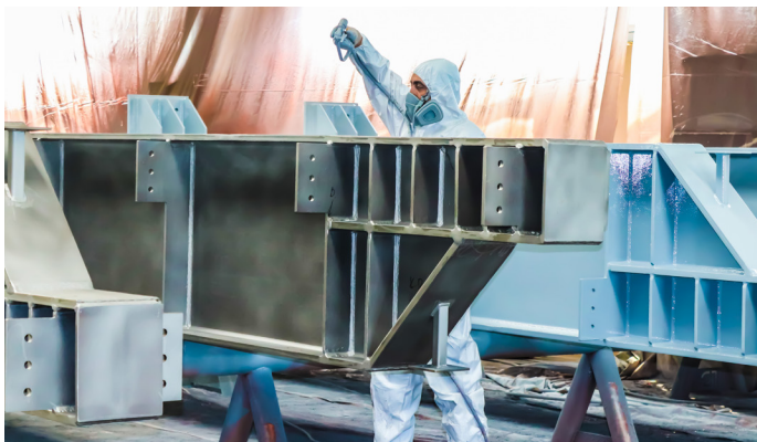
Figure 1. Shorter primer cure windows are where many two-coat schedule gains start – organic zinc primers can cut that waiting time significantly in shop-applied bridge steel.
