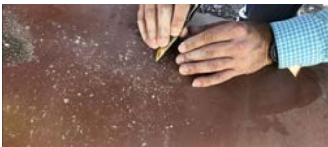
Figure 2. Rock drop testing proved that a chemical composite fusion-bonded epoxy (FBE) overcoat provides the impact and abrasion resistance required to protect the base anti-corrosive FBE layer from becoming exposed.
