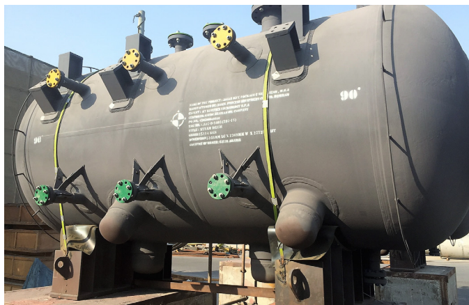
Figure 4. An MIO-embedded IMM coating can effectively mitigate CUI when applied to process vessels operating at high temperatures and covered with insulation.
