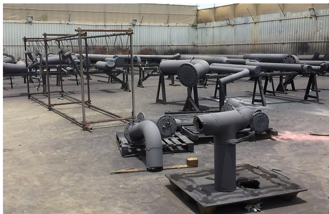
Figure 2. Applying coatings embedded with micaceous iron oxide (MIO) to large pipes and valves can effectively protect those assets from damage and corrosion prior to service, as well as mitigate the effects of CUI when assets are later insulated and placed into service.
