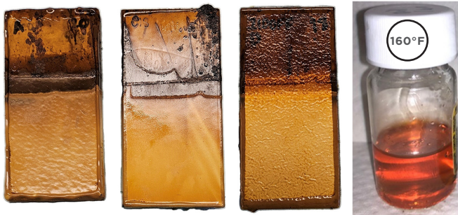
15 months exposure in vegetable oil (+DI water) at 160°F [71°C]
