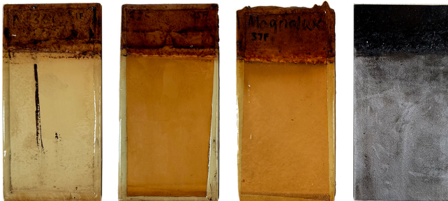
Vegetable oil and water – eight months cyclic exposure at 180°F [82°C]
