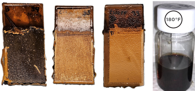
15 months exposure in vegetable oil (+DI water) at 180°F [82°C]
