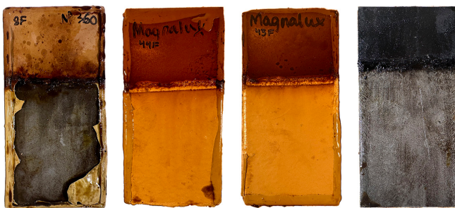
Vegetable oil and water – six months exposure (no cycling) at 180°F [82°C]
