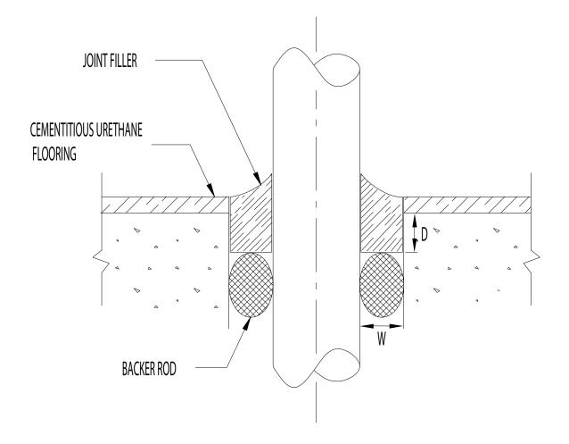
D = W/2 D = DEPTH OF BACKER ROD W = WIDTH OF JOINT
