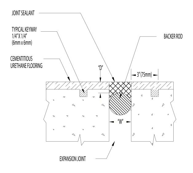
D = W/2 D = DEPTH OF BACKER ROD W = WIDTH OF EXPANSION JOINT
