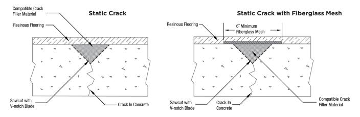
Prior to filling static cracks, be sure to prepare them by removing all laitance, debris and sealers. Make a sawcut with a V-notch blade attached to a vacuum.
