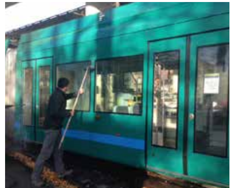
AFTER: Rather than take the rail car out of service for several days to strip and repaint this rail car, was cleaned with the GRS non-toxic solution and back in service within two hours.
